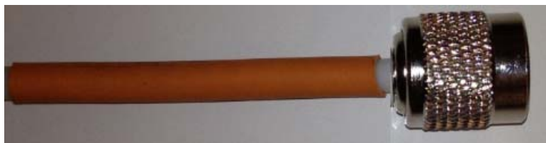
Figure 31: Cable Installation, with Allowance for Connector
